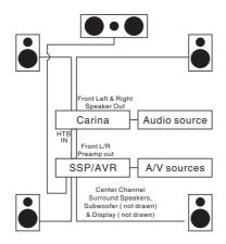
Connect Line-level (RCA style) front left and right outputs from the AVR or SSP to the ANALOG input on the Carina.
