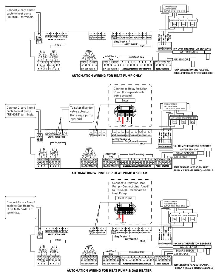
Figure 14: Automation Connections
