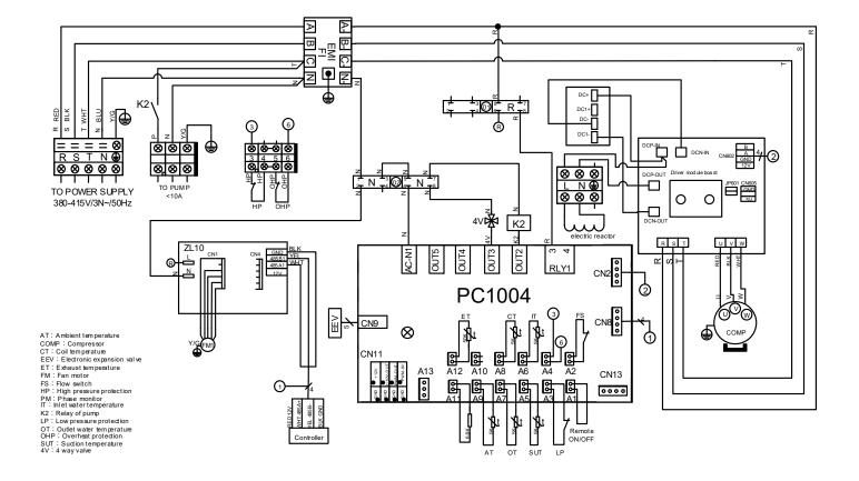
Figure 17: Wiring Diagram - UltraTemp 28kW HXi models
