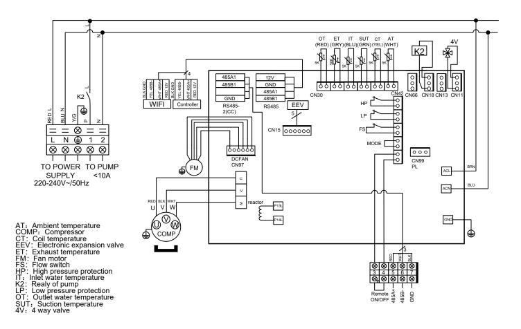
Figure 15: Wiring Diagram - UltraTemp 9kW & 12kW HXi models
