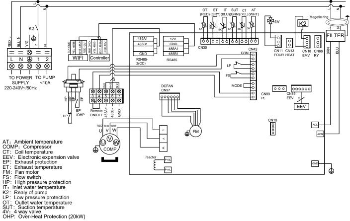
Figure 16: Wiring Diagram - UltraTemp 16kW, 20kW & 24kW HXi models
