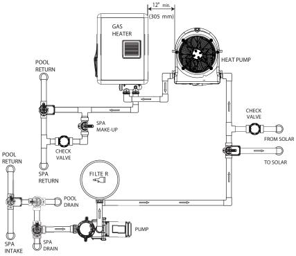
Figure 8: Multiple Heat Source Configuration
