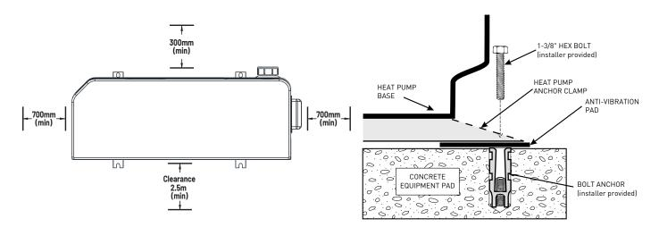
Figure 3: Anchor Clamp Installation
