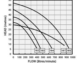
Horizontal, single stage, surface mounted centrifugal pump with closed impeller for pumping debris free water coupled to a cool running Totally Enclosed Fan Cooled 2 pole motor.
