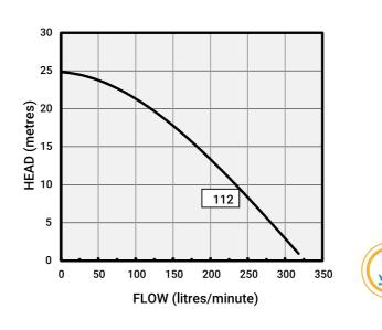
Horizontal single stage, surface mounted centrifugal pump with closed impeller for pumping debris free water coupled to a cool running Totally Enclosed Fan Cooled 2 pole motor with external thermal overload (single phase only, three phase units require separate quick trip overload supplied by electrical contractor).
