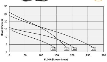
Horizontal single stage, surface mounted centrifugal pump with closed impeller for pumping debris free water coupled to a cool running Totally Enclosed Fan Cooled 2 pole motor with thermal overload protection.
