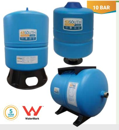
A pressure tank is an essential part of a pressurised water system that provides water pressure at a set level. The tank stores supplemental water between diaphragm and liner. This process reduces the number of times the motor needs to start in order for the system pressure to remain at the set level.
