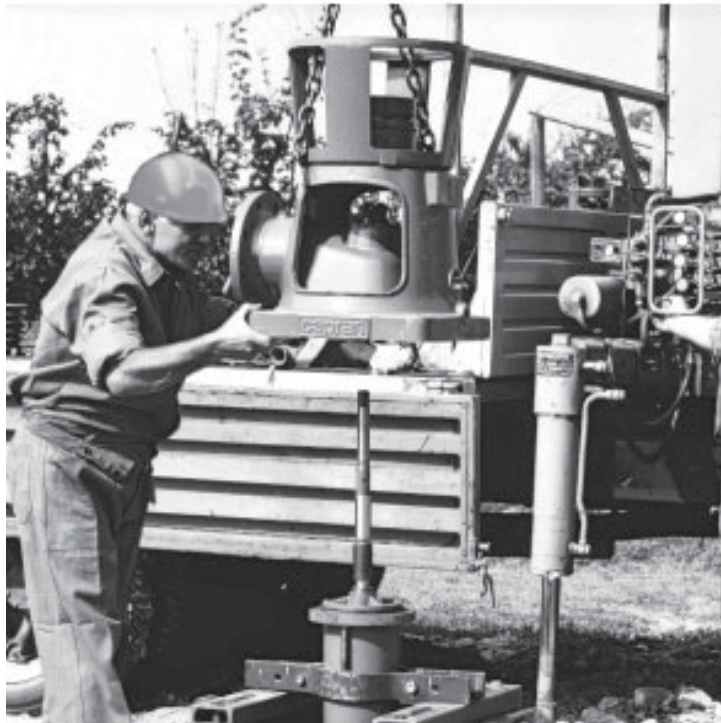
fig. 15 - Lower the control unit after having made sure that it is perfectly aligned
