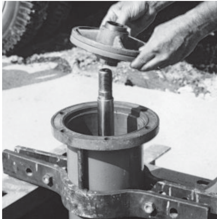
fig. 8 - Fit the rod support into the pipe housing
