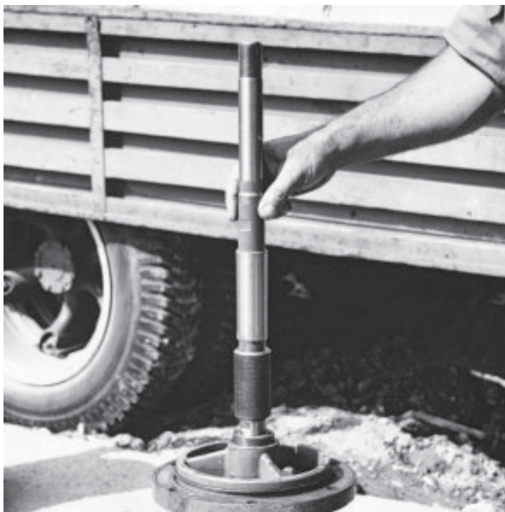
fig. 14 – Screw in the connection shaft and lock the threaded sleeve
