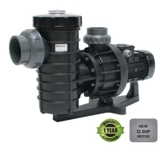
PENTAIR Thermoplastic Centrifugal Pumps are self priming, single stage, close-coupled (Pump with built-in electric motor, with the motor drive and pump impeller on the same shaft), monoblock centrifugal pumps with closed impeller and mechanical seals.
