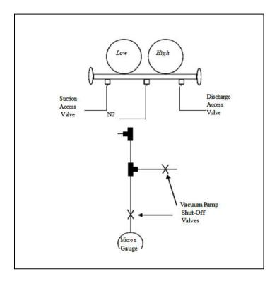
**Figure 1.** Manafold connections for Vacuum pump and Electronic Micron Gauge
