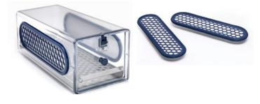
The replaceable 0.2  $\mu$ m membrane filter has an effective pore size of about 0.02  $\mu$ m when filtering air<sup>1</sup> and is hydrophobic, oleophobic, resistant to organic solvents and tested for biosafety and low cytotoxicity.
