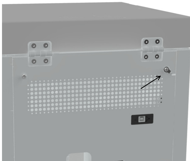
Figure 4. Opening chamber cover in emergency
