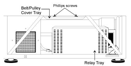
Figure 4-9. Front View of Cabinet with Grille Removed
