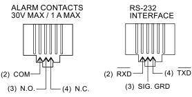
Figure 1-15. RS-232 and Remote Alarm Connectors
