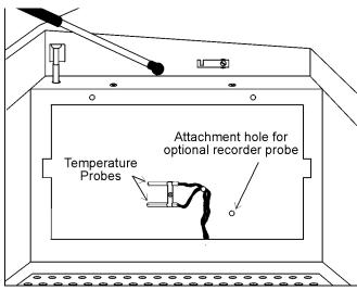
Figure 4-5. Right Side Chamber - Temperature Sensor Cover Plate Removed
