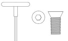
Figure 1-8. T-Handle Wrench and Hex Socket Head Screw
