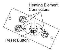
Figure 4-8. Heating Element Connectors and Manual Reset Circuit Breaker
