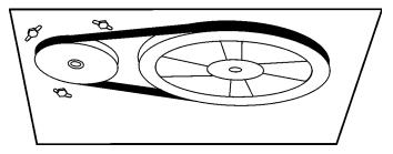
Figure 4-10. Motor/Belt Drive System
