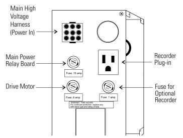
Figure 4-3. Fuse Holder and Connector Locations (SHKE481HP shown)
