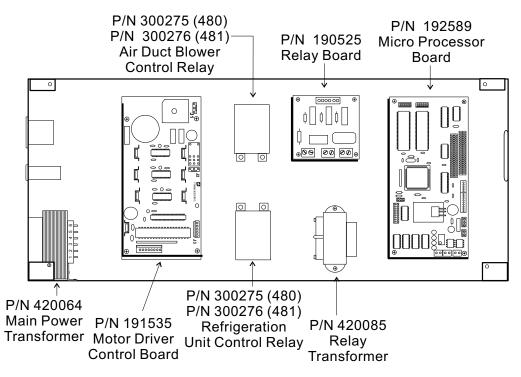
Figure 4-4. Electrical Component Locations, Relay Tray Compartment
