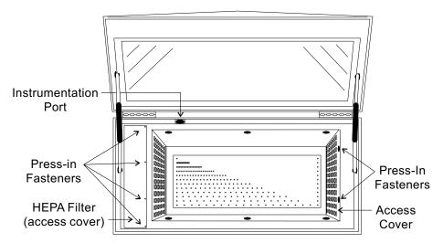
Figure 4-1. HEPA Filter and Temperature Sensor Locations
