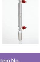
Liebig condensers are used to cool and condense hot vapor as part of a distilling apparatus. This condenser has a straight inner tube that the condensing vapor passes through, and a larger outer jacket that cooling water passes through. Socket
