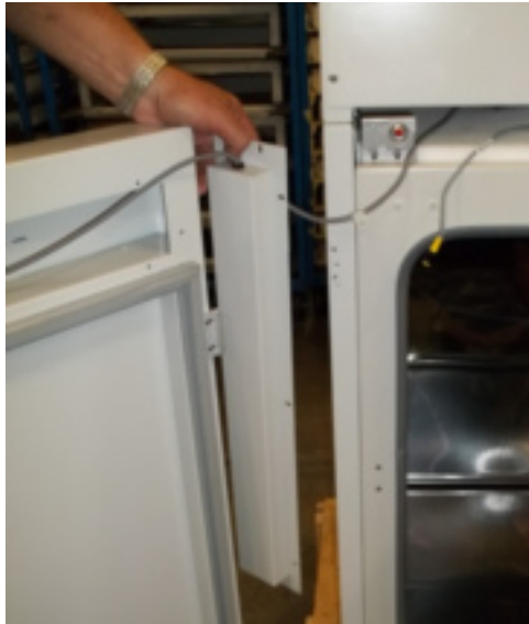
Figure 6-11. Set Door and Pan Aside
