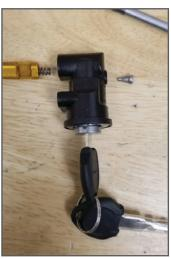
Reassembly is the reverse of disassembly; hold the lock assembly in the bicycle downtube with the key, replace the upper battery receptacle and orient the lock assembly so the orange latch pin inserts through the hole in the battery receptacle. Reinstall the 2 short screws for the lock assembly, then replace the 1 long and 2 short screws holding the receptacle into the bike downtube.
