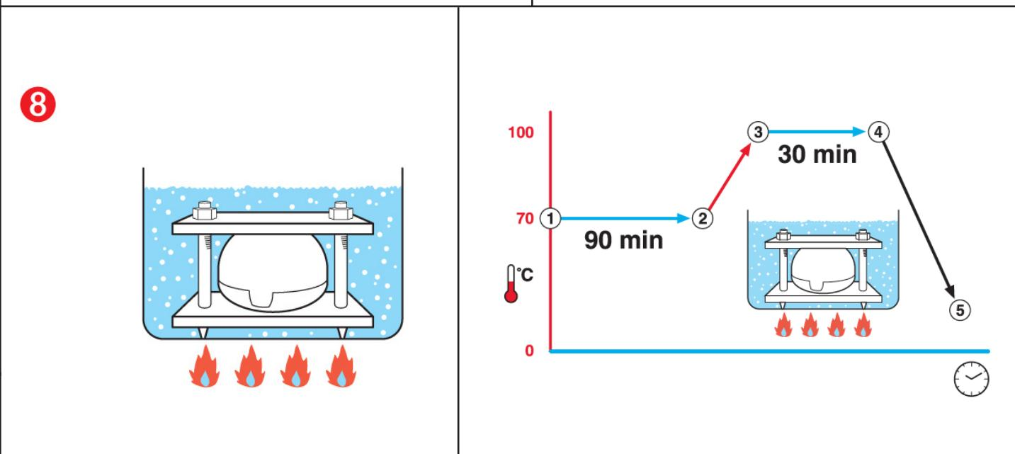
**En** - ① Start curing process in hot water + Maintain water temperature ② Increase water temperature ③ Start curing + Maintain water temperature ④ Stop curing + Air cooling to ambient temperature ⑤ End of total curing process
