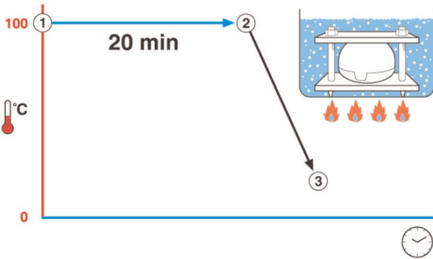
**En** - 1). Start curing process in hot water + Maintain water temperature. 2). Stop curing + Air cooling to ambient temperature . 3). End of total curing process.
