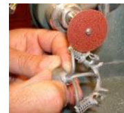
Cut-off and Finishing Partial Frames
