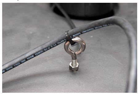
Use provided zip-tie to secure light power cable to eyebolt. The power cable should not have any stress on the first light fixture. Connect the end of the power cable to the supplied transformer and enjoy the show.
