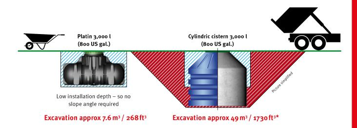
\* Based on a vertical, cylindric cistern with a useable volume of 3,000 l (800 US gal.), a height of 1.90 m (6' 3") and a diameter of 2.20 m (7' 3") Calculation of excavation is under consideration of a ditch bottom of 10 cm (4"), a sidewise distance of 50 cm (19.7") and a slope with 45° gradient according to DIN 4124.
