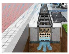
Combination of filtration channel and a filter media- professional solution for handling polluted surface water runoff.
