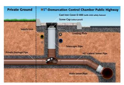
\*600 mm radius to allow entry of maintenance equipment
