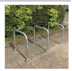
The VELOPA Sheffield Cycle Toastrack is a floor fixed cycle rack based upon the Sheffield Cycle Stand. The Sheffield Cycle Toastrack consists of Sheffield Cycle Stands welded at 800mm centres to floor fixed box section rails. The benefits of a Cycle Toastrack over individual stands are reduced installation costs and pre-determined gaps between stands, each stand is suitable for parking two bicycles. The Sheffield Toastrack is ideal where cycle parking in large numbers is required.
