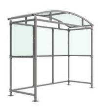
The Inglewood shelter is a free-standing, open fronted shelter designed for on site assembly, constructed from galvanised mild steel. Complete with a 4mm UV stabilised PETG clear sheet roof, and ½ side panels. Side-to side curved roof.
