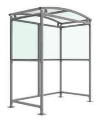
The Burbank shelter is a free-standing, open fronted shelter designed for on site assembly, constructed from galvanised mild steel. Complete with a 4mm UV stabilised PETG clear sheet roof, and ½ side panels. Side-to side curved roof.
