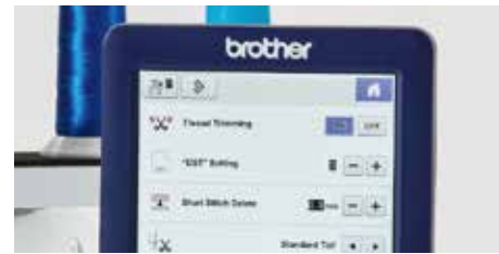
Automatic thread cutter Cuts upper and lower thread automatically at the end of each colour change on embroidery.
