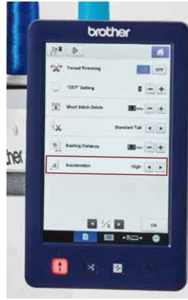
Industrial level acceleration Complete embroidery designs now even faster – reach maximum embroidery speed in just 7 seconds. After thread trimming, the machine will reach max. embroidery speed quickly. The acceleration is comparable to industrial embroidery machines.
