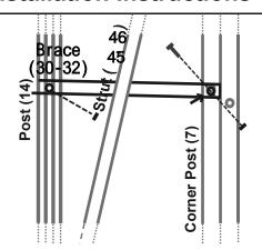
**Note:** All Braces are installed inside the Posts, but outside the Struts. See diagram above, shown from inside the greenhouse facing out.
