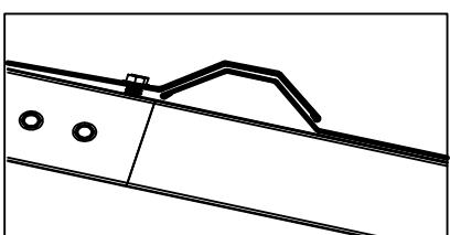
Color steel tile connection should pay attention to the above a piece of pressure below a piece, to prevent water
