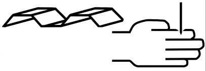
Care must be taken when handling various pieces of your building since many contain sharp edges. Please wear work gloves, eye protection and long sleeves when assembling or performing any maintenance on your building.
