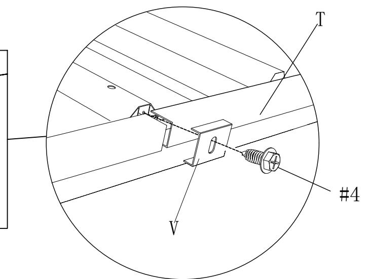
When assembling each colored steel tile(GG), pls note to fix using the longer plate(T) and shorter plate(V) immediately to prevent the tile sliding. Safety is important!
