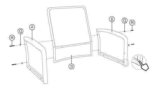
Locate the Chair Seat(C) to the Armrests(A & B) by the pre-drilled threads. Fasten Bolts(M) with Washers (Q) by usin g Allen Key(R) to combine armrests and chair seat together.
