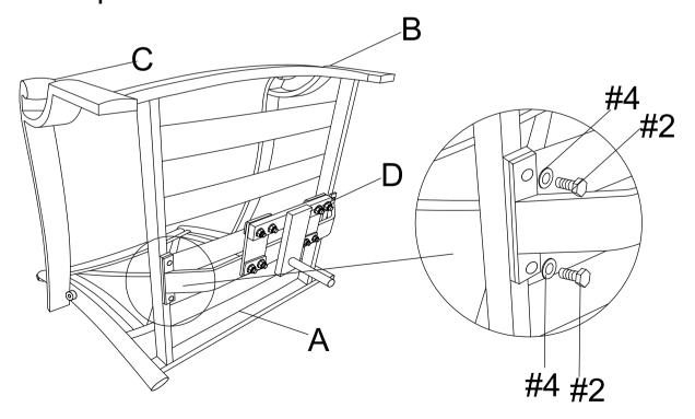
DO NOT TIGHTEN SCREWS UNTIL ASSEBMLE IS DONE!
