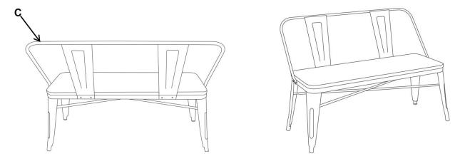
Step 3 - Insert one Bolt (Part E) through each of the bolt holes in the BACK and into the threaded inserts in the Seat Top. Do not tighten first. Tighten all bolts holes after bolts in place.
