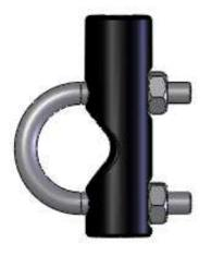
2. Place the Low Profile Mounting Block on the tube you want to mount it too. Place the "U" bolt through the 2 holes on either side of the "V" of the Mounting Block.
