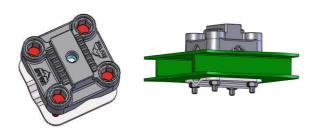
**Extended Position: DO NOT** use the supplied washers! This will allow the hex bolts shown in red below to drop further down into the mounting block. The mounting block will now fit round tubes up to 1 1/2", square tubes up to 1 1/4", and composite (plastic racks) up to 1 1/4" thick.
