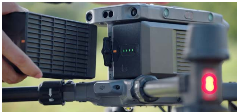
Figure: Battery hot-swapping
