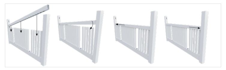
10 Push mid rail into slot on 1 post then lever into slot on adjacent post. Insert pickets as the mid-rail is levering down. Posts may flex to allow for insertion.
