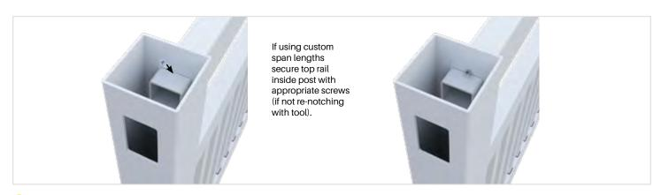
If using custom lengths, re-notch the tongues with notching tool (sold separately) or secure top rail in place on post using appropriate screws.
