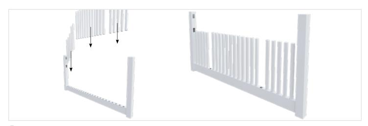
9 Install short pickets into bottom-rail leaving long pickets for subsequent step. The long pickets are postitioned 6 pickets in from either end.
