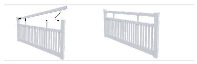
12 Install top rail over long pickets guiding pickets into holes on underside of top rail. Insert top rail into one post and then lever into adjacent post.
