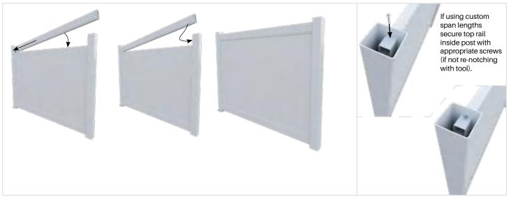
Install top rail over vertical panels and simultaneously push top rail as far as possible into one post and then slide back into adjacent post. Standard length top rails are self-securing using the pre-notched tongues.
