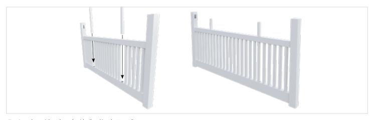
Insert long pickets through mid-rail and into bottom rail.
