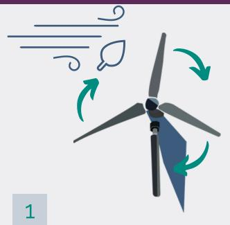
Fast blowing wind holds the energy to make the turbine blades rotate.
