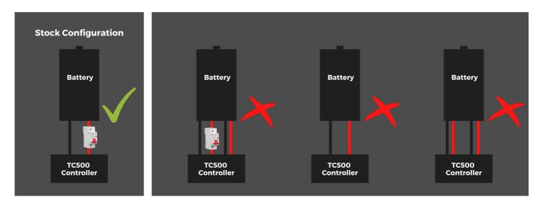
Use only tools and screws that came with the controller. Using the tools and screws that were not included in the parcel, not following these instructions, or not using the fuse, can cause serious damages to you and your bike.
