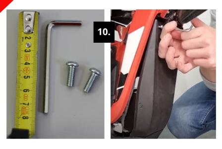
**STEP 10:** Use the longer M6 screws and a larger hex key to fasten the shield to the frame.
