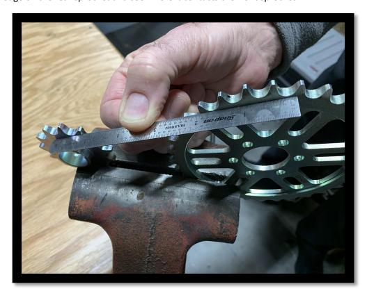
If the alignment gap at the front sprocket is off by more than 1mm, add or remove the shim to bring it back into alignment. Some bikes using the 420 kit will require the alignment shim and some will not. The 219 kit seem to not need it for two reasons: 1) We designed it in house to fit without the use of a shim and 2) Due to many more links the 219 will accept more misalignment without the excessive noise and wear. Always check the alignment when installing your kit.
