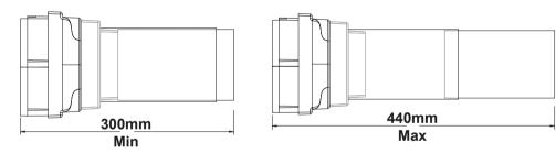
**2.** Extend the telescopic pipe to suit the width of the cavity wall and needs of the extractor system being installed.
