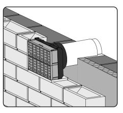
**1.** Build the **thru...air** product into the masonry as it proceeds. The product must be installed angled slightly down towards the external brickwork to allow for any condensation build up to drain out via the Airbricks.
