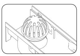
**4.** Once the channel is installed, fit the Leaf Trap into the outlet hole which has been created.
