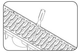
**8.** To remove the grate, use a flat blade screwdriver at the clip points to ease the clips open. The grate can be further secured using 4  $3.5 \times 30$ mm self tapping screws.
