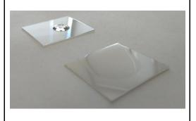
Two pieces of polycarbonate were plasma treated to clean and hydroxylate the surfaces. The cleaned polycarbonate was dip-coated with CytoSyl and air cured at room temperature for 60 minutes. The picture shows 100 microliters of mineral oil on each of the pieces. The CytoSyl coated piece is "repelling" oil and the uncoated piece is "attracting" oil.
