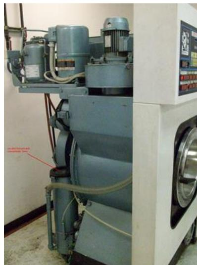
Depending on results, determine if the tips are dry, if not increase the heat and chill steps. The goal is to recover the maximum amount of solvent while also coating the tips with polymer.
