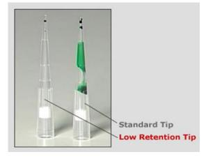
FluoroPel low retention polymer coatings are a great choice to reduce error when pipetting buffers, surfactants, viscous liquids and other materials. FluoroPel coated tips improve pipetting accuracy, save reagent costs and make experimental work more reproducible. The goal of this paper is to introduce the methods used for coating tips with FluoroPel.
