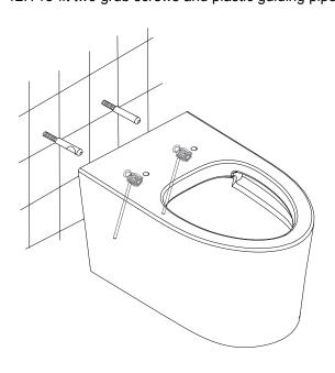
13. Install the toilet on to fixing bolts. Then tighten the grub screws.
