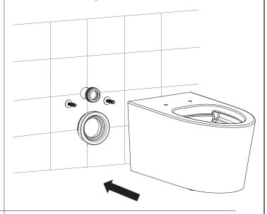
10. Fit the fixings into wall hung holes. Fixing bolts on WC frame (not supplied).
