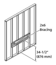
To properly support the weight of the vanity and basin, secure to stud framing or 2x6 bracing behind the finished wall.
