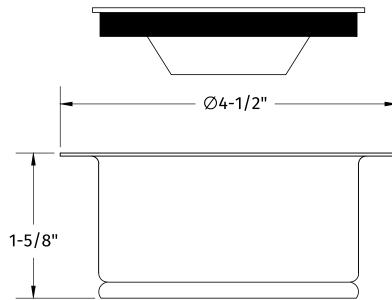
WILL FIT STANDARD Ø3-1/2" DRAIN **OPENING** FOR USE WITH CONTINUOUS FEED **3-BOLT MOUNT DISPOSERS WITH** 3-3/8" I.D. SOLID STOPPER FOR SEALING WATER FITS SINKS UP TO 5/8" THICK COMPATIBLE WITH **MOUNTAIN PLUMBING 3-BOLT** MOUNT **INSINKERATOR** FRANKE 3-BOLT MOUNT **KENMORE** WHIRLPOOL **KITCHENAID** MOEN
