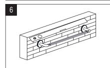
Temporarily place the towel bar on the mounting brackets to check alignment. If necessary, loosen the screws and realign the mounting brackets.
