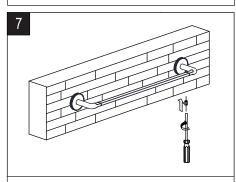
Place towel bar assembly on the mounting brackets. Secure it to the wall using the bottom set screws.
