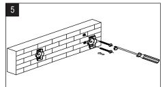
Place the mounting brackets over the wall anchors. Secure them to the wall using the supplied screws.
