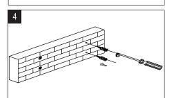
Drive the wall anchors into the drilled holes with a Phillips screwdriver.
