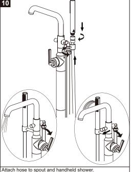
Once hand shower is attached turn on TUB FILLER and test the diverter
