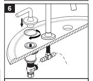
Place the "O"ring over the valve. Place the handle assembly on the valve. Secure the assembly by turning the handle hub clockwise.
