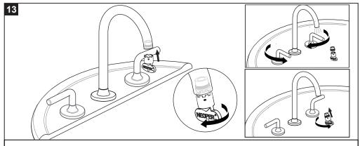
Remove aerator with key and flush out debris. Reinstall aerator and save aerator key for homeowner.
