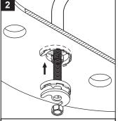
Slide "C" washer up on supply tube.
