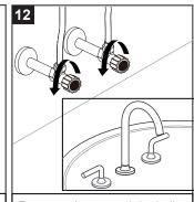
Turn on angle stops and check all connections for leaks.
