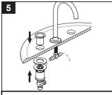
Push valve up from the bottom and thread on the valve sleeve from the top to secure the valve. If the deck is less than 1 3/8" thick use the supplied spacer. If the deck is thicker than 1 3/8" do not use the spacer.
