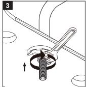
Carefully tighten spout nut to secure spout.
