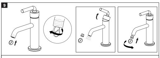
Remove aerator with coin and flush out debris.
