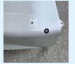
Drill 7/8" hole/install grommet in both sides of front cover
