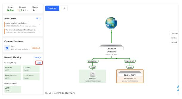
Method 2: Click manage in the Network Planning area on the Overview page to go to the Network Planning page for configuration (Network >> Network Planning). Click Add Wi-Fi VLAN to add the Wi-Fi VLANs to the live network or select the available Wi-Fi VLANs.
