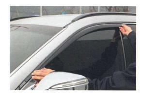
Once you are satisfied with the alignment, carefully peel off the backing from the tape and install....IMPORTANT: it's essential to get this correct first time as reattempting this will make the tape ineffective.
