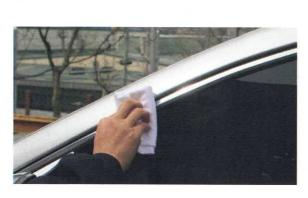
2. Use sachet A to clean the attachment area, we have provided two, one for each side of the vehicle. Allow 10 minutes to dry.
